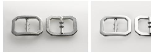
Belt buckle before and after processing in an OTEC disc finishing machine
