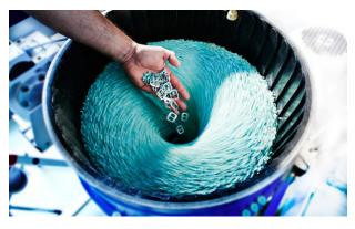
Intensive processing through different centrifugal forces
