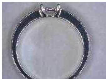
Intricate silver ring after two-stage mechanical processing (Ra \mu\text{m} 0.030). Source: OTEC.
